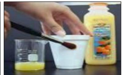
8) The lemon juice was spread on the side of a Styrofoam cup with a brush, and the observation was recorded in the next five minutes.
